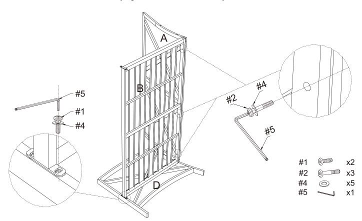
Step 3. Attach right arm panel (part C) to back panel (part A) and seat panel (part B) using short bolts (part #1), long bolts (part #3), flat washers (part #4) and allen wrench (part #5).
